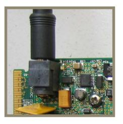
Connect the 12V DC power adapter (supplied with the kit) to power jack (J6).
